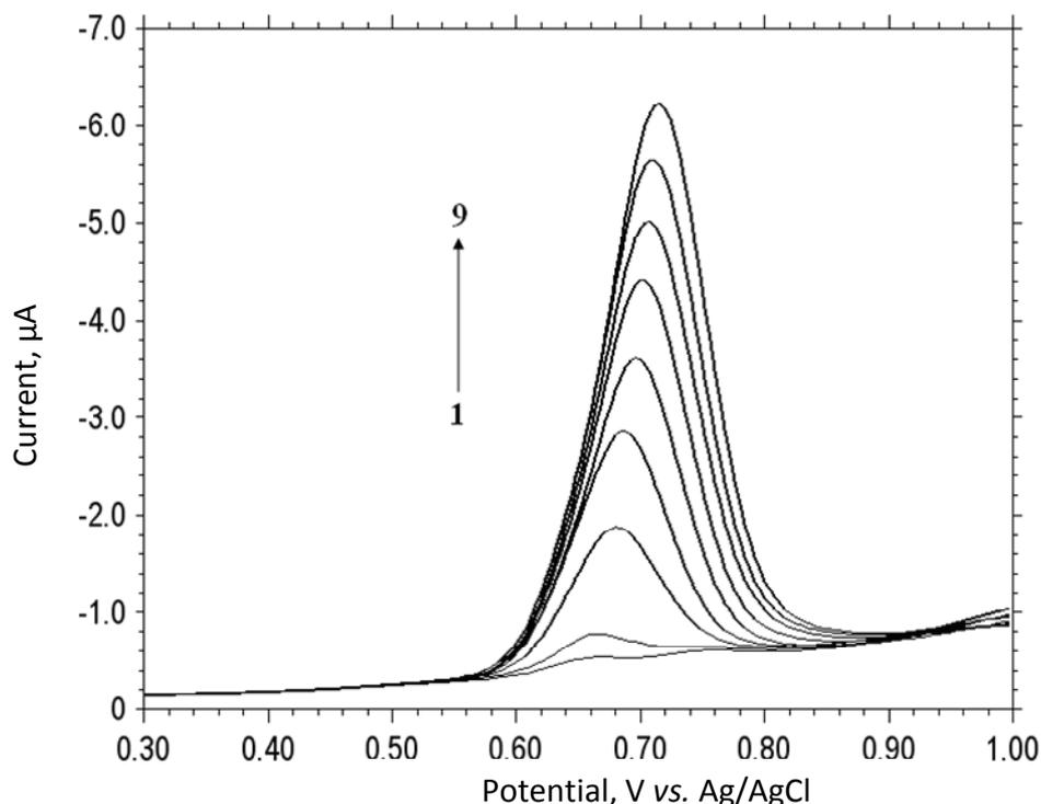
**Figure 5.** Differential pulse voltammograms for increasing concentrations of NVP in phosphate buffer at pH 10 at a GCE. Scan rate:  $10 \text{ mV s}^{-1}$ ; pulse amplitude: 50 mV; and pulse width: 30 ms. NVP concentration was maintained at (1) 5.0, (2) 10, (3) 50, (4) 100, (5) 150, (6) 200, (7) 250, (8) 300, (9) 350  $\mu\text{M}$ .
